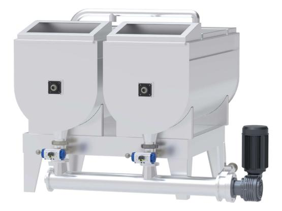
Introduction: Malaxation machines are mixing tanks in which olive paste is gently kneaded. Thanks to specially designed mixing blades, cell walls are broken down, improving oil extraction efficiency and aroma development. These tanks help oil droplets coalesce and prepare the paste for decanter separation. **Application:** The malaxation stage plays a critical role in both **oil yield and quality**.
